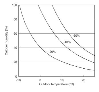
Condition; Model:FTXR50EV1B Indoor temperature setting:20°C Airflow rate:Max Room volume:120m³ Air change rate:0.5/hour humidifying hose length:7.5m
