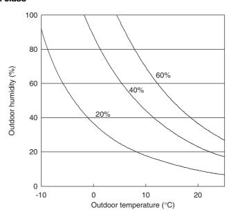
Condition; Model:FTXR42EV1B Indoor temperature setting:20°C Airflow rate:Max Room volume:100m³ Air change rate:0.5/hour humidifying hose length:7.5m
