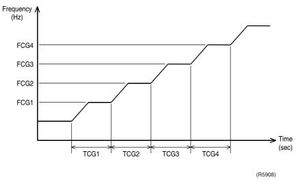
Fig. : Compressor protection function graph.
