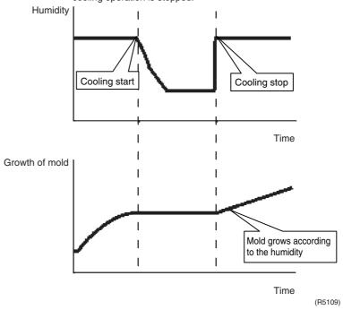
Mold shock operation after cooling The humidity in the room is lowered suddenly by Mold Shock Operation.
