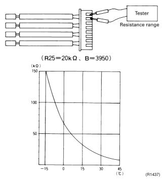
■ For the models in which the thermistor is directly mounted on the PCB.
