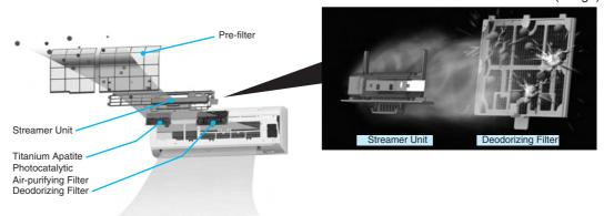
Powerfully decompose and remove molecules of allergens or odors by collision with high-speed electrons discharged from streamer unit.
