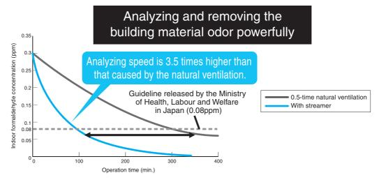
The formaldehyde concentration in the laboratory (10 m²) at 0.5-time ventilation and the initial concentration setting of 0.3 ppm (Observed by Daikin using the FTXR28E) (Nozaki laboratory, Graduate Course of Health and Society System, Tohoku Bunka Gakuen University)
