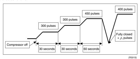
Fig.: Pressure equalization control graph in cooling mode
