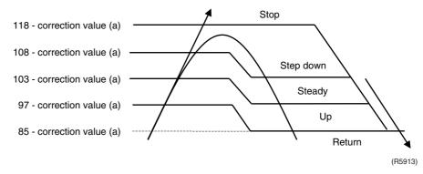
Correction value (a) = correction value by operation frequency (b) +correction value by outdoor temperature (c)
