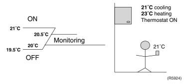
Between the indoor unit and the position of the end user, there is taken into calculation a temperature shift of 0.5°C. This means that at thermostat OFF, the temperature at the end user is e.g. 20°C.
