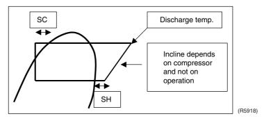
Fig.: Target discharge pipe temperature control graph
