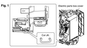
Remove the remote controller lid and cut the address jumper "J4". (See Fig. 2)
